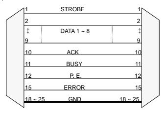
25 Pin D-SUB Connector (FEMALE) Printer 25 Pin D-SUB Connector (MALE) HOST
